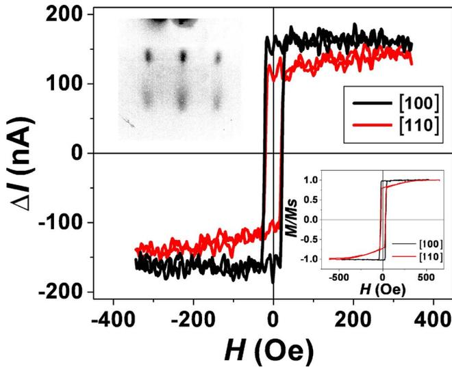
FIG. 1. (Color online) Magnetic field dependence of  $\Delta I$  for a sample with an epitaxial Fe/GaAs(001) interface using a photon energy of 1.96 eV. The sample was measured at zero bias and along different magnetic field directions. The observed RHEED pattern for the Fe layer along the [110] direction and MOKE loops for the same sample are shown in the inset.
