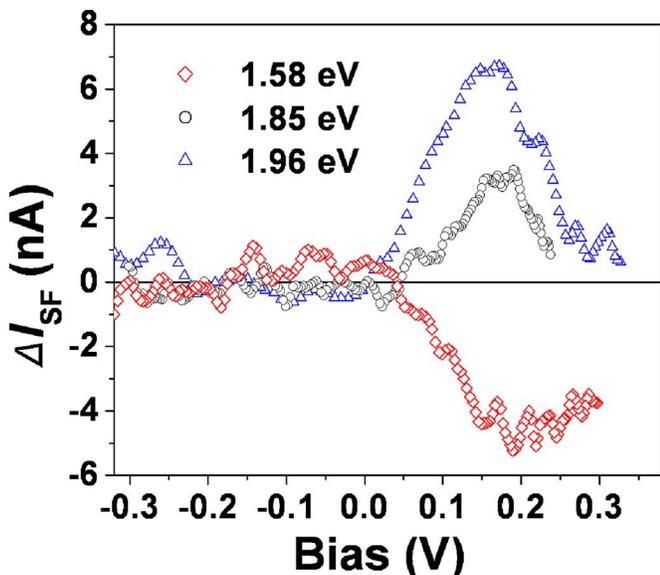
FIG. 2. (Color online) Bias dependence of  $\Delta I_{SF}$  for an epitaxial Fe/GaAs(001) interface for different photon energies.
