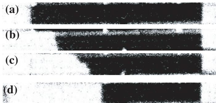
**Figure 9.** PMOKM images for the [110]-oriented device at 102 K, showing the domain wall position and profile after applying single current pulses of current density (a)  $6.0 \times 10^5$ , (b)  $6.2 \times 10^5$ , (c)  $6.75 \times 10^5$  and (d)  $8.0 \times 10^5$  A cm<sup>-2</sup>.
